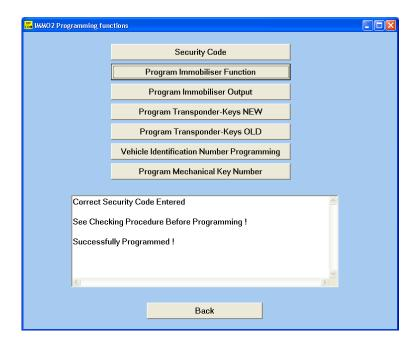
When you replace both Engine and Immobiliser ECU, both programming routine will be executed after each other. First, the Immobilser ECU will be programmed with the Secret Code, VIN, and MKN, then a new Engine ECU will be adapted to the system.
